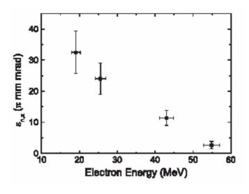
Figure 3: Nomalized vertical emittance  $\varepsilon_{n,x}$  as a function of electron energy.
