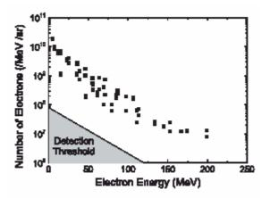
Figure 2: Electron energy spectra for  $2.5 \times 10^{19}$  cm<sup>-3</sup> electron density and a laser irradiance of  $3 \times 10^{18}$  W/cm<sup>2</sup>. An effective longitudinal electron temperature of  $(18 \pm 1)$  MeV can be derived for electrons of less than 130 MeV (continous line).
