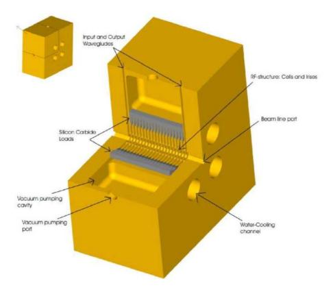
Fig. 2 Schematic geometry of the HDS structure
