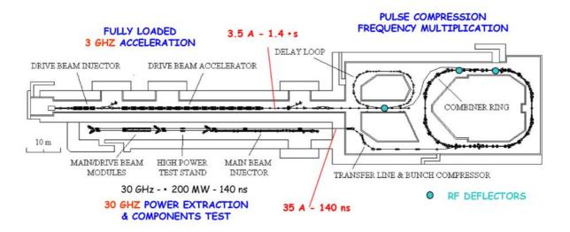
Fig.1 Scaled Layout of the test facility CTF3
