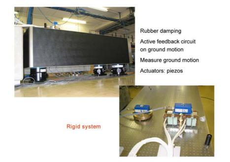
Fig. 5 CLIC vibration test stand
