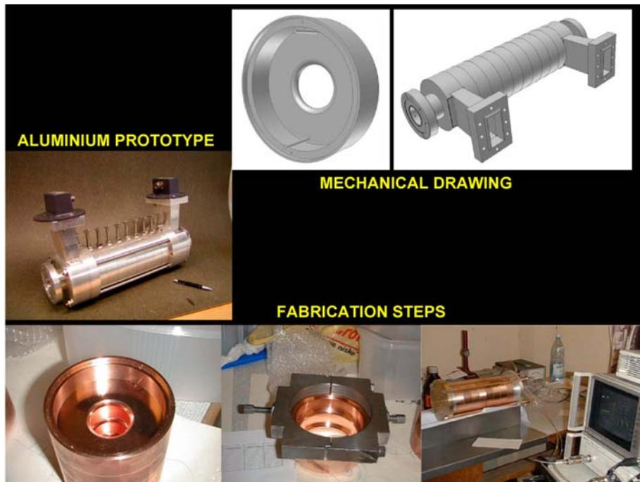
**Fig. 6 Prototype of the CTF3 RF deflector.**
