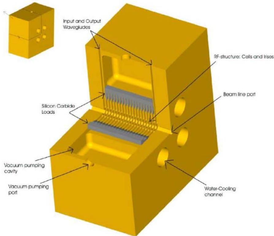
**Fig. 2 Schematic geometry of the HDS structure**
