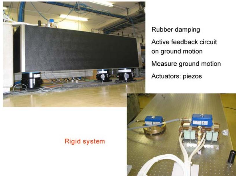
**Fig. 5 CLIC vibration test stand**
