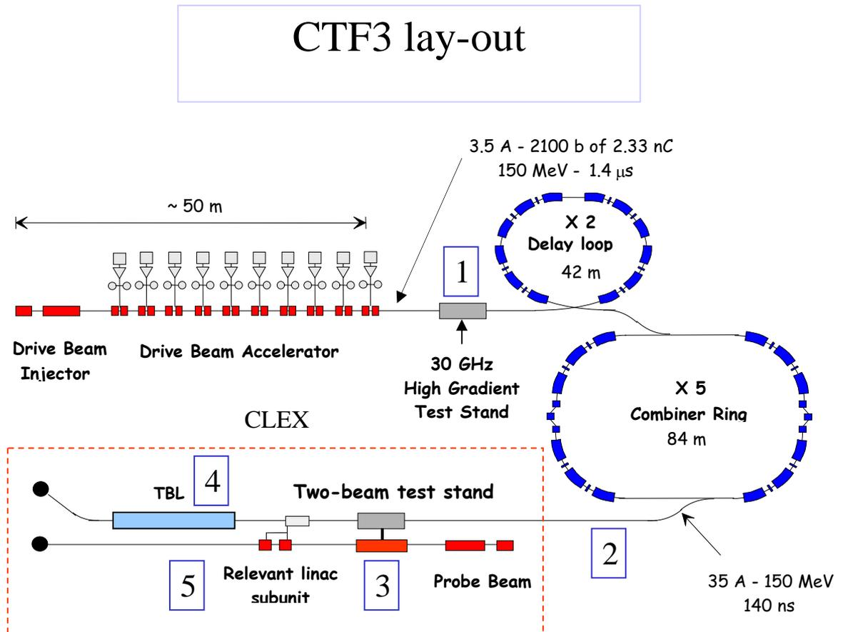
**Fig. 7 Schematic layout of the CLIC Test Facility CTF3**
