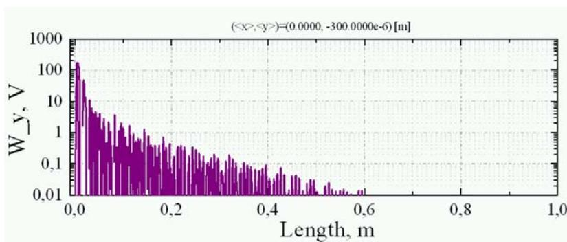
**Figure 6: Transverse wakefields of the structure in Fig. 5.**
