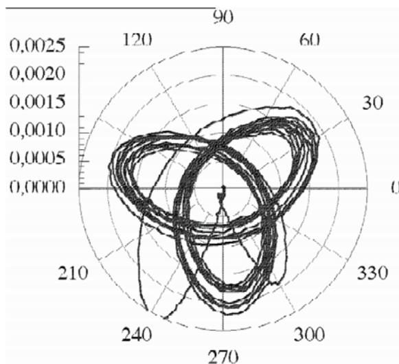
**Figure 2: Polar chart of the  $2\pi/3$ -mode from a bead-pull measurement.**
