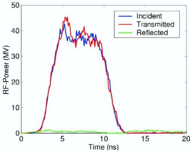
**Figure 3: Typical measured incident, transmitted and reflected RF pulse during**
