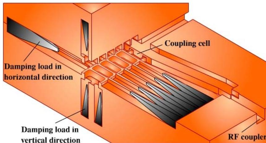
**Figure 5: Structure with loaded waveguides in horizontal and vertical direction.**
