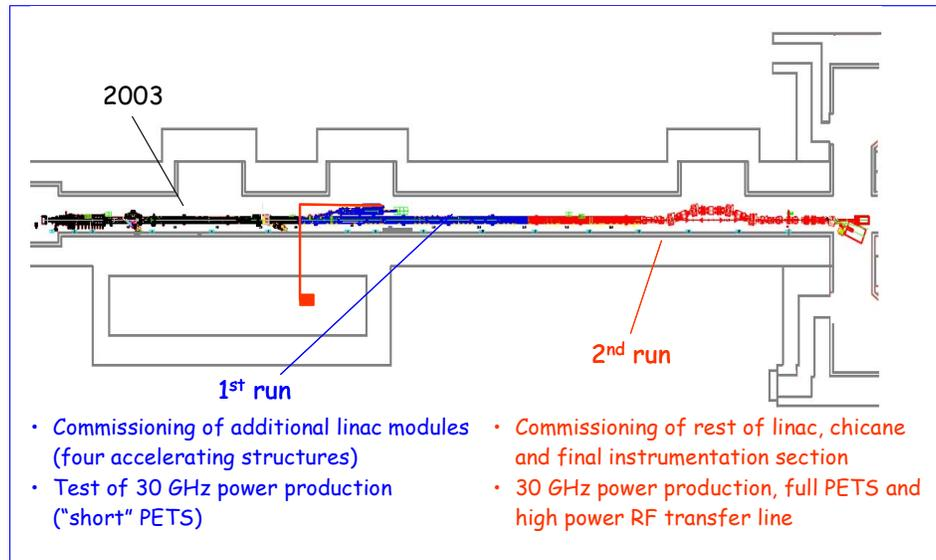
Fig 4: Layout of the CTF3 linac, describing beam operation in 2003 and 2004.
