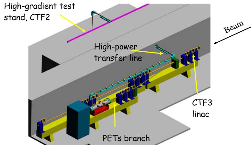
Fig 3: New “PETS Line” installation and 30 GHz RF power transfer line to the test area
