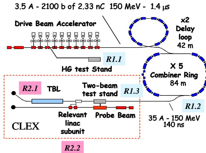
Fig 1: Layout of CTF3 with the main building blocks
