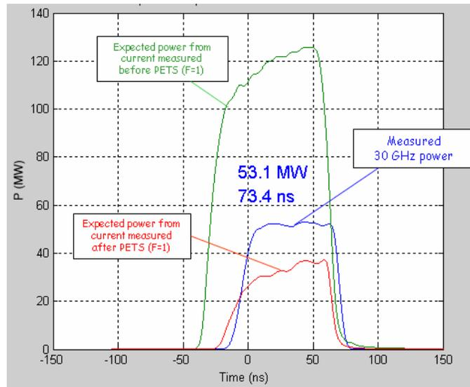
Fig 5: Results of power production test.
