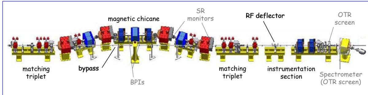
Fig 6: The INFN chicane and the end-of-linac instrumentation region.
