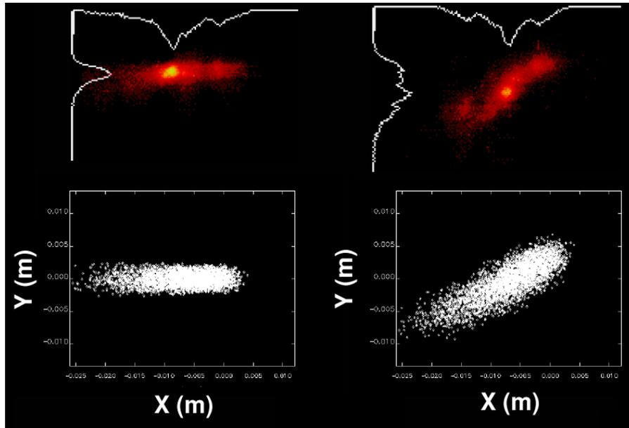
Fig 7: Measured (top) and simulated (bottom) beam transverse beam distributions with the RF deflector off (left) and on (right), for  $R_{56} = 0.1$  m. Horizontal dispersion at the location of the screen is responsible for the correlation visible in the images to the right (from C. Biscari, INFN/LNF).
