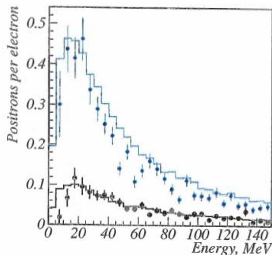
Figure 4: Positron energy distribution (from R. Chehab / LAL)
