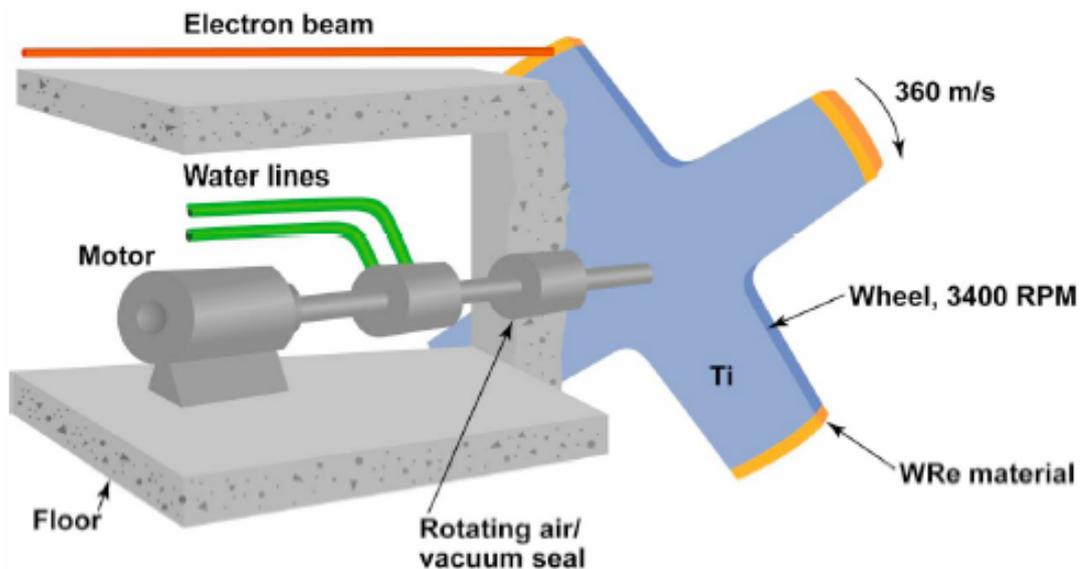
Figure 3: Conventional source target system layout (from W. Stein et al. / LLNL)
