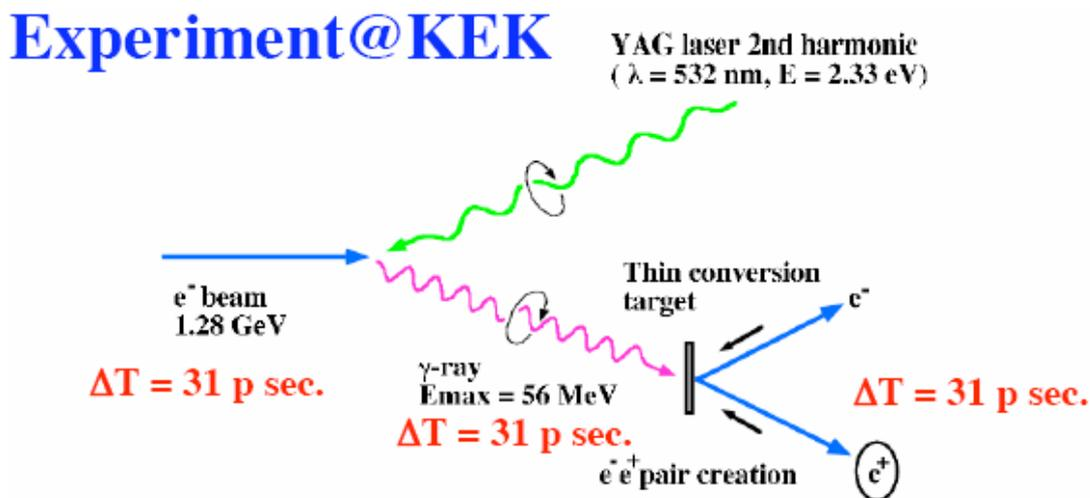
Figure 5: Layout of Laser back scattering for proof-of-principle demonstration (from M. Kuriki/KEK)
