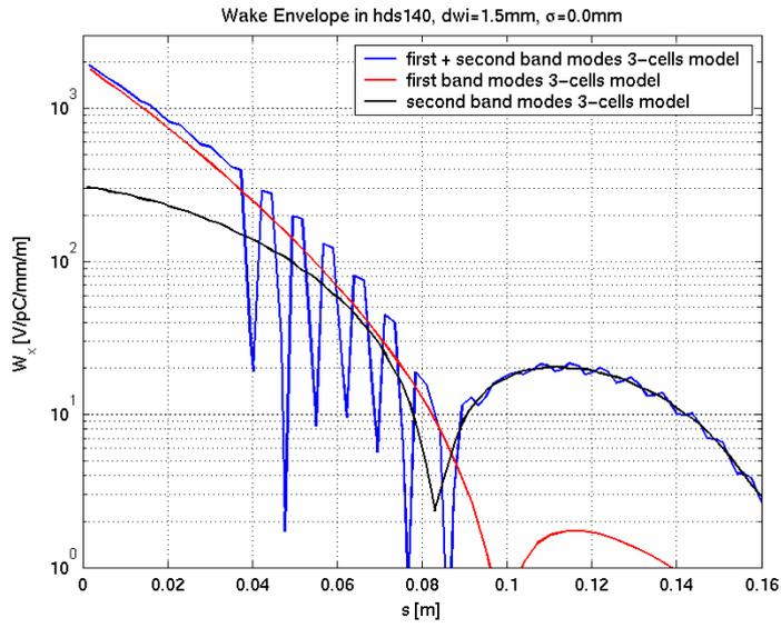
Fig3. Calculated wake-field envelope, for the HDS structure.
