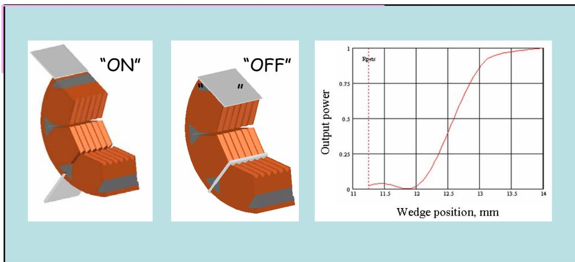
Fig.5 Sketch of the wedge system developed to switch on/off the power generation of a transfer structure.
