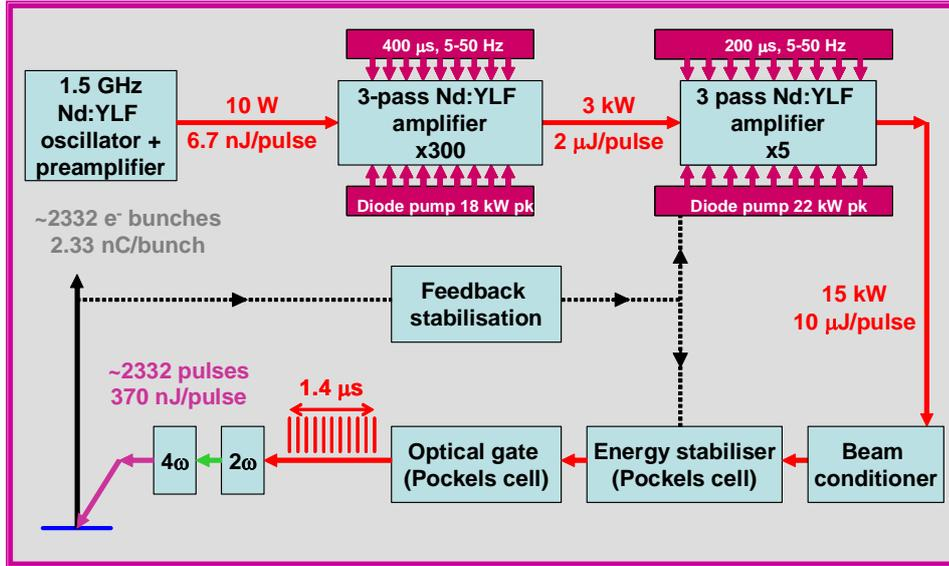
Figure 5: CTF3 Laser system (Courtesy of M. Divall-RAL)
