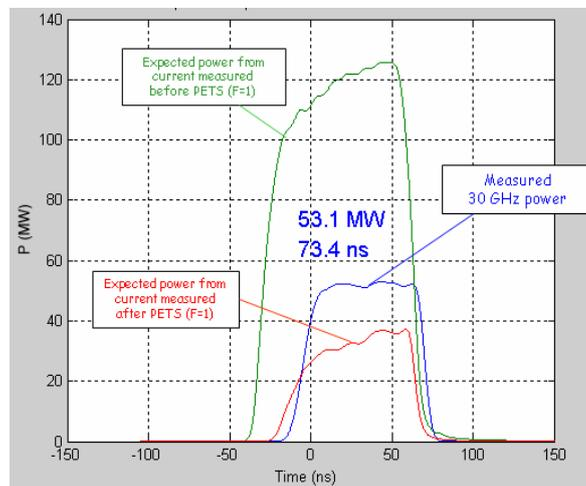
Figure 4: Results of 30 GHz RF power production test (in a load)
