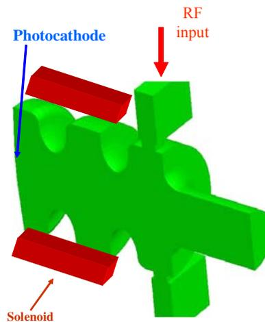
Figure 8: Model of the RF gun (Courtesy of R. Roux –LAL)
