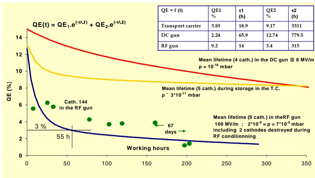
Figure 7: Quantum efficiency versus time (Courtesy of G. Suberlucq-CERN)
